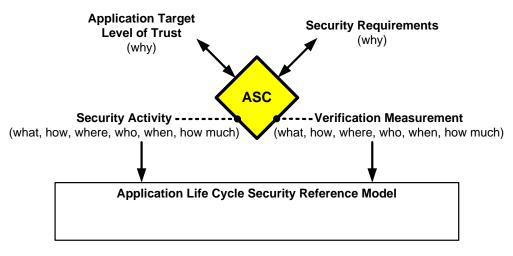
Figure 6 – Components of an ASC
